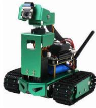
Fig. 6. We implement our algorithm on Nvidia Jetson intelligent toy car.
